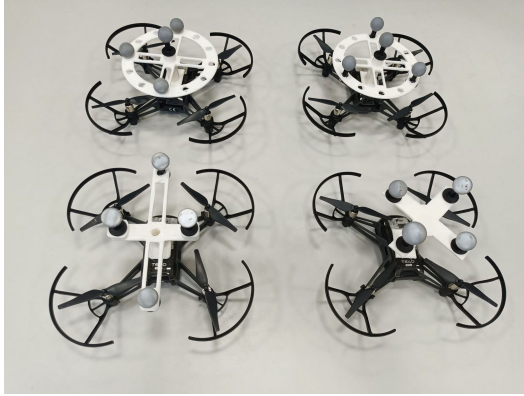
Fig. 13. Tello UAVs with marker attachments.
