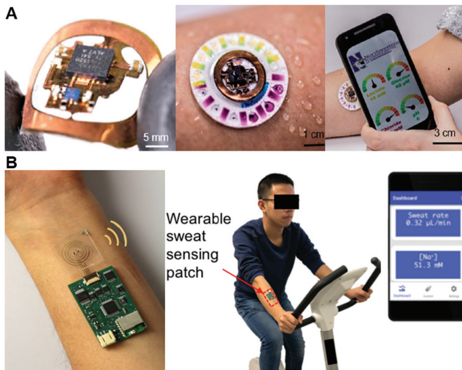
Figure 12. Wireless data transmission. A) NFC. Reproduced with permission. [72] Copyright 2019, AAAS. B) Bluetooth. Reproduced with permission. [101] Copyright 2018, American Chemical Society.
