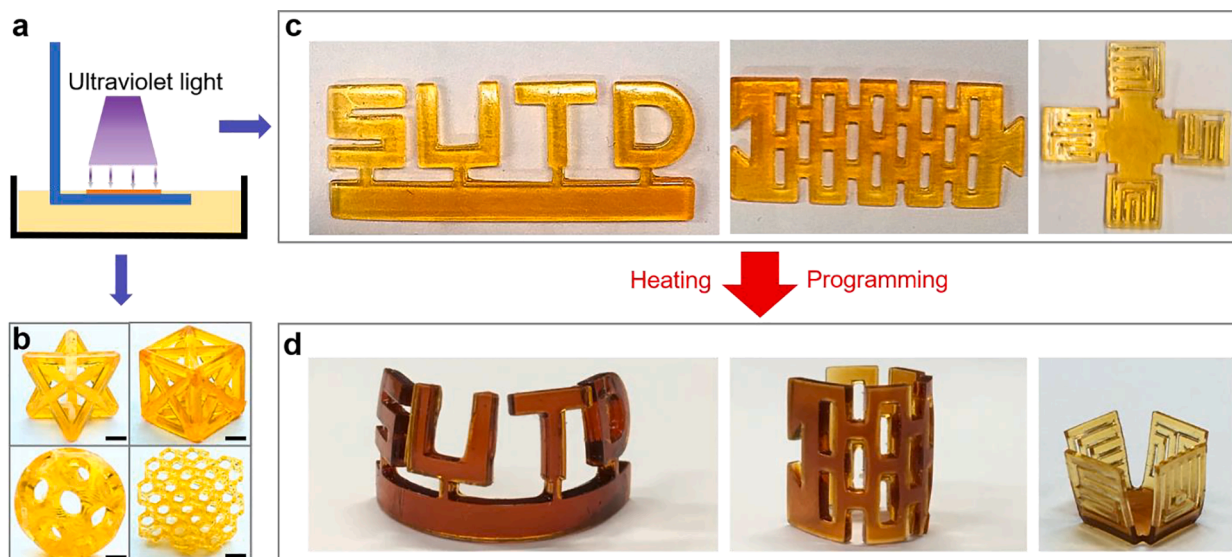
Fig. 4. 3D printing of dual-curing polymer network system. (a) Scheme of DLP apparatus. (b) Demonstration of printed structures. The scale bars all represent 2.0 mm. (c, d) Examples of programming printed 2D sheets into permanent 2.5/3D structures through dual-stage processing.
