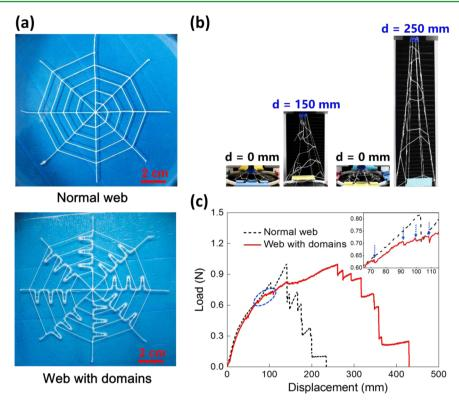
Figure 4. (a) Photos of printed network structures mimicking spider-webs: a normal web versus a web with folded domains. (b, c) Snapshots at certain displacement, d, (b) and force—displacement curves (c) of the two structures in a. The arrows in the inset of c indicate the breaking events of sacrificial bonds that lead to the unfolding of individual domains.
